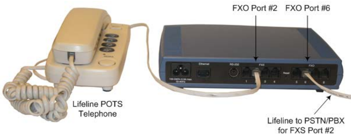
Figure 5-10: Lifeline Cabling for FXS and FXO Devices
