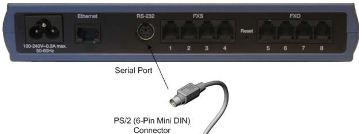
Figure 5-13: Connecting the Serial Port
