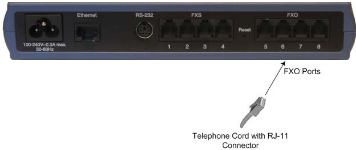
Figure 5-7: Connecting FXO Interfaces
