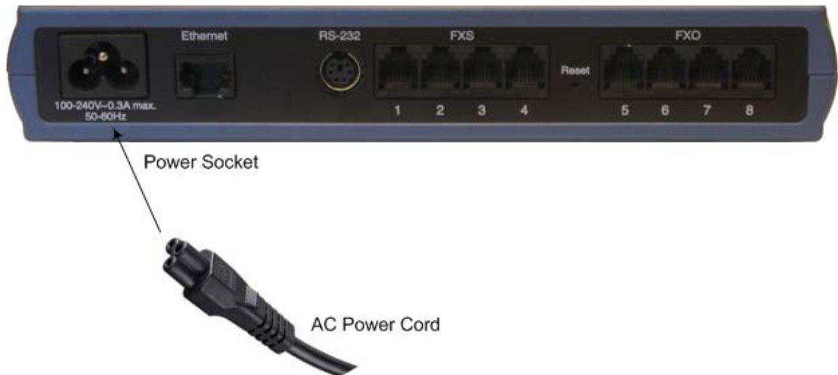
Figure 5-14: Connecting to the Power Supply
