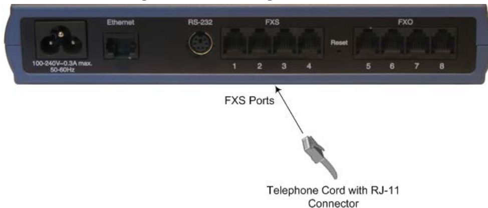
Figure 5-5: Connecting FXS Interfaces
